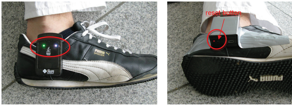
Figure 9: Sun SPOT acceleration sensor mounted on a shoe.
